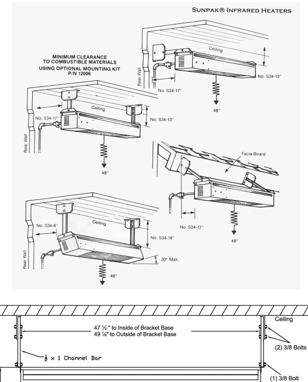
Warning: Heater must be level in the lengthwise direction.
