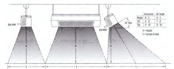
SUNPAK will raise the comfort level 5-10° Fahrenheit outdoors. The above coverage table was based on still breeze conditions. Under windy conditions more heat will be required. It is recommended that a windswept patio be designed with wind breaks to stabilize the patio environment. Wind breaks shall NOT interfere with the ventilation or combustion air requirements of the heater(s) and meet clearance for combustible requirements listing on page 6 & 7.
