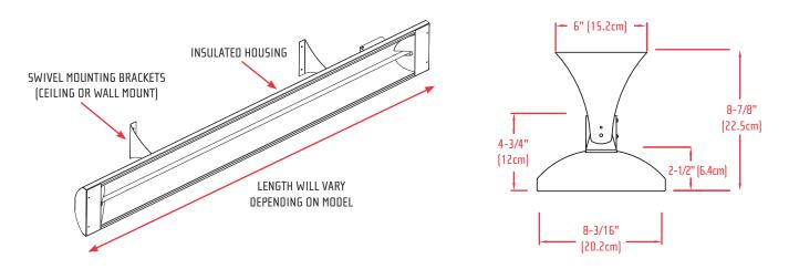
Heater must be installed with the quartz tube horizontally level. For maximum tube life, use a carpenter's level tool to find the optimum level position for the heater's body. It's important to always maintain the minimum clearances from the heater body to any combustible materials.
