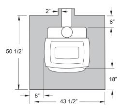
Figure 10. Floor Protection minimum dimensions, Canada.
