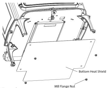
Figure 24b. Bottom Heat Shield installation
