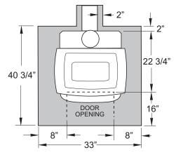
Figure 9. Floor Protection minimum dimensions, U.S.
