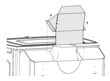
Figure 2. Flue Collar heat shield attachment.
