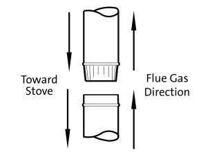
*Figure 3. Chimney connector orientation.*
