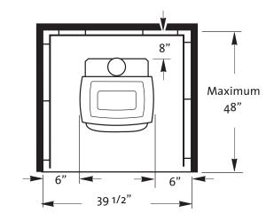
Figure 12. Alcove with Wall Protection.
