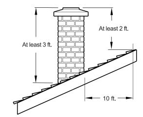
Figure 4. Chimney Height Requirement.
