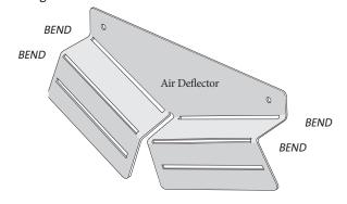
Figure 19. Air Deflector orientation.
