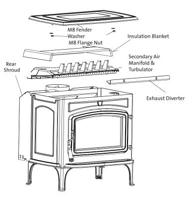
Figure 26. Overview of secondary air manifold removal
