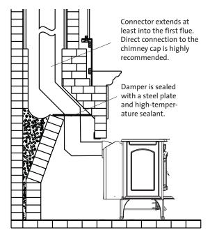
Figure 7. Hearthmount Installation.
