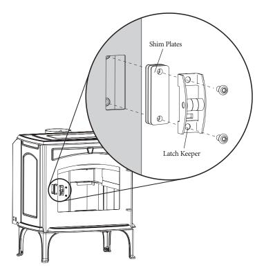
Figure 17. Latch adjustment.
