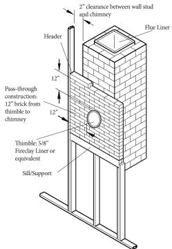
Figure 5. Masonry Wall Pass-through.
