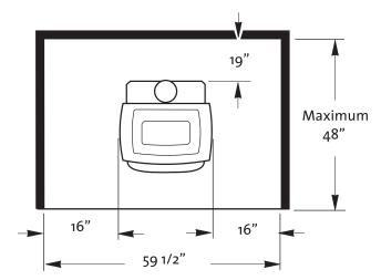
Figure 11. Alcove with Unprotected Walls.
