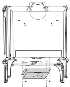
Figure 23. Outside Air Adaptor installation.
