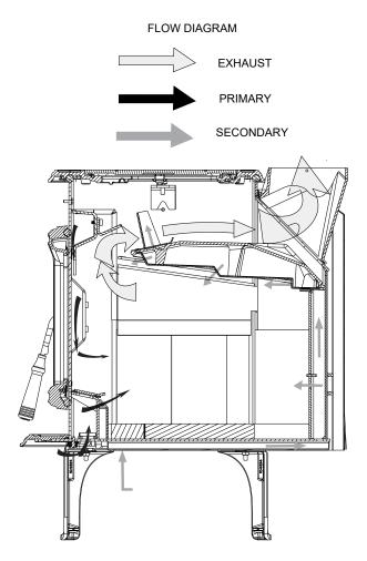
Figure 15. Combustion air paths
