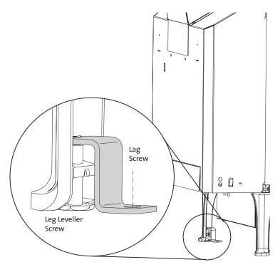
Figure 25. Floor Bracket Detail
