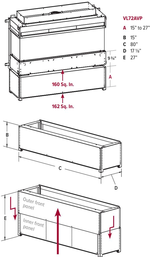
NOTE: the fireplace chase must be vented both above and below appliance, no fans are required.
