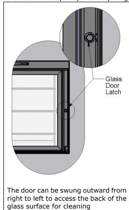
Figure 4 Glass Door Latch Pin
