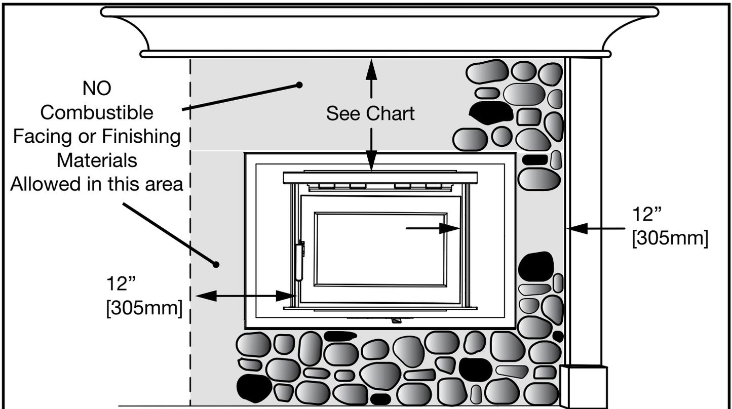
Figure 23: FP16 LE Facing Material Clearances.
