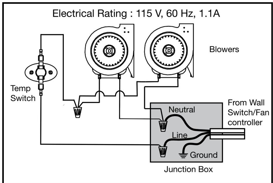
Figure 17: FP Wiring Diagram.
