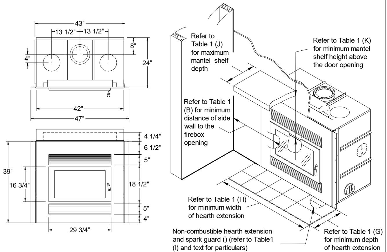
**Figure 1 Unit Dimensions and Clearances**
