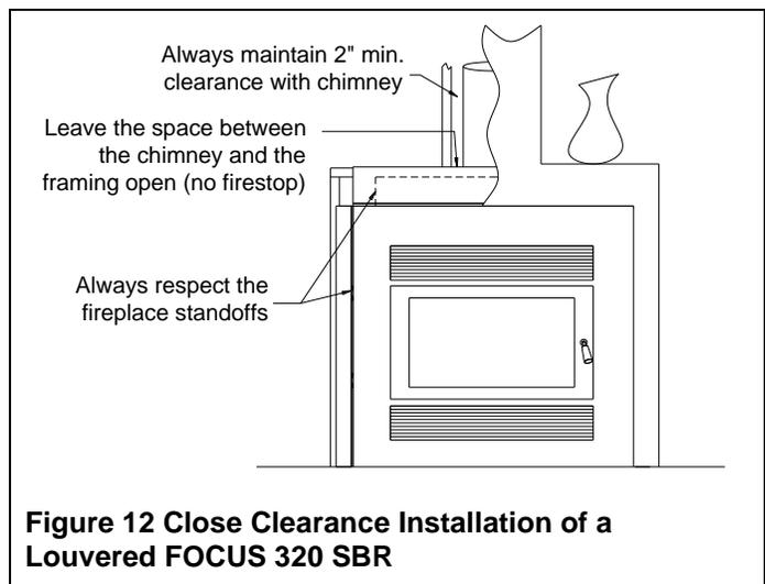
**Figure 12 Close Clearance Installation of a Louvered FOCUS 320 SBR**
