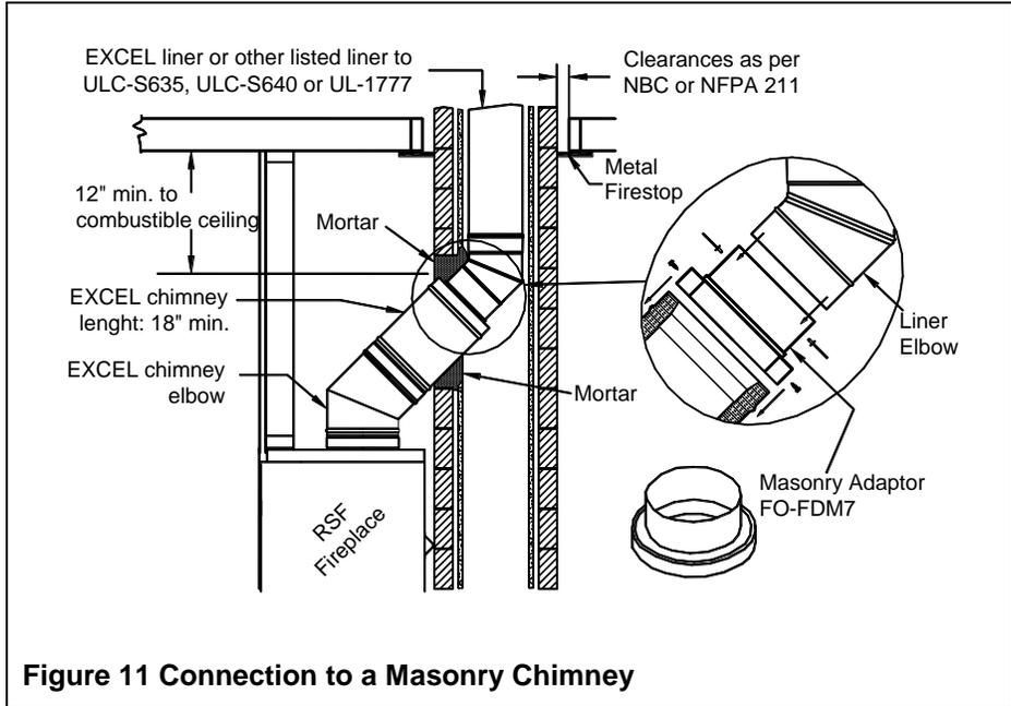
**Figure 11 Connection to a Masonry Chimney**
