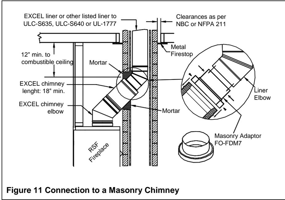
**Figure 11 Connection to a Masonry Chimney**
