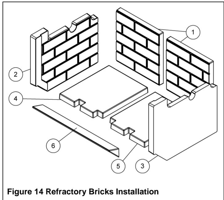
**Figure 14 Refractory Bricks Installation**
