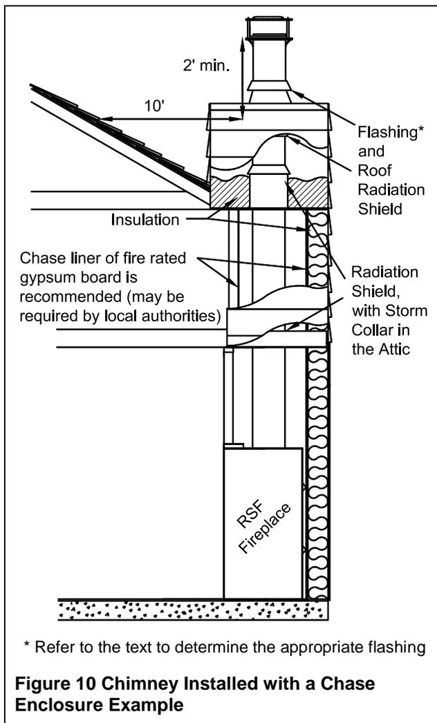
**Figure 10 Chimney Installed with a Chase Enclosure Example**
