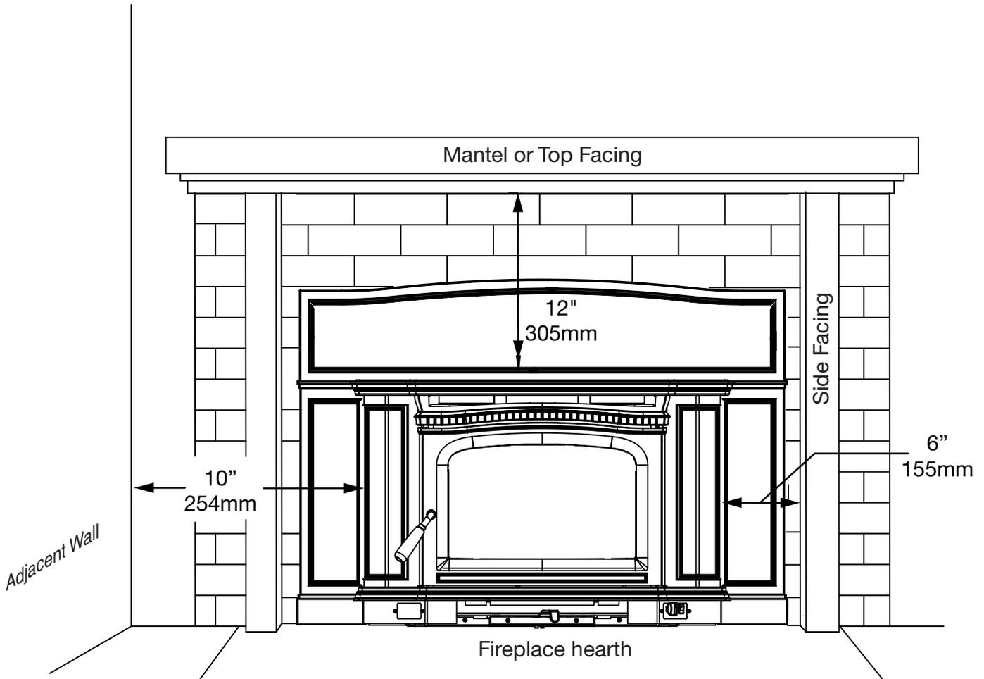
Figure 5: Clearances - ALT 5 Insert LE.
