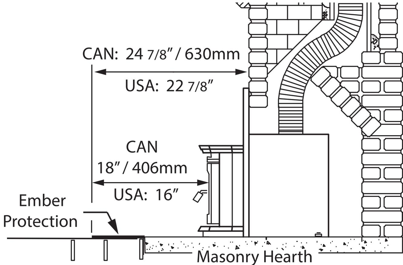
Figure 4: ALT5 Insert LE - Ember protection.
