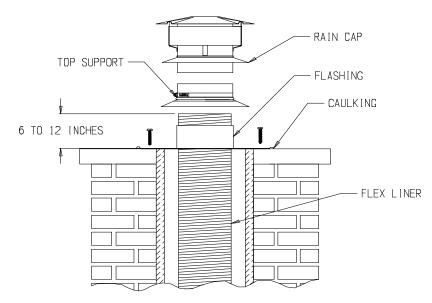
Cap into the liner. Tighten up on gear clamp supplied on Top Support crimping liner onto the Rain Cap base allowing it to overlap the flashing collar preventing any rain from getting between flashing collar and liner.
