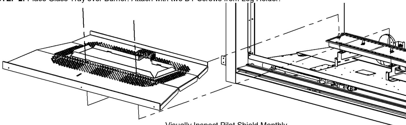
Visually Inspect Pilot Shield Monthly for signs of deterioration due to flame exposure. Replace if necessary.
