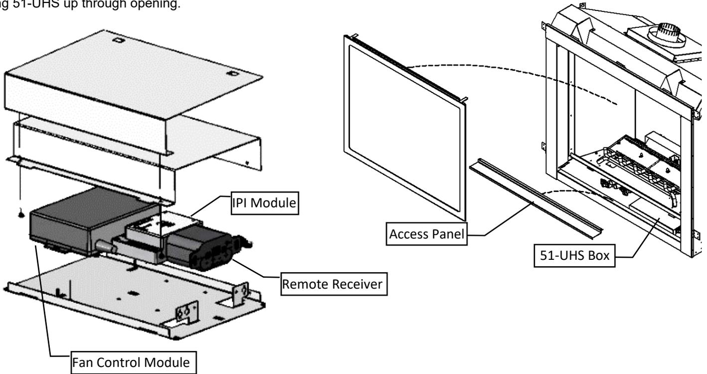
51-UHS can be inserted & removed from beneath fireplace through access panel opening (Remove glass door first).
