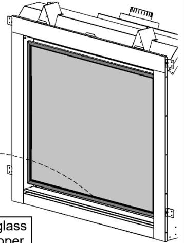
To install screens hook bottom clip onto glass door frame, then press down and push upper clip under top glass door frame, then release. Clip will hook onto frame.
