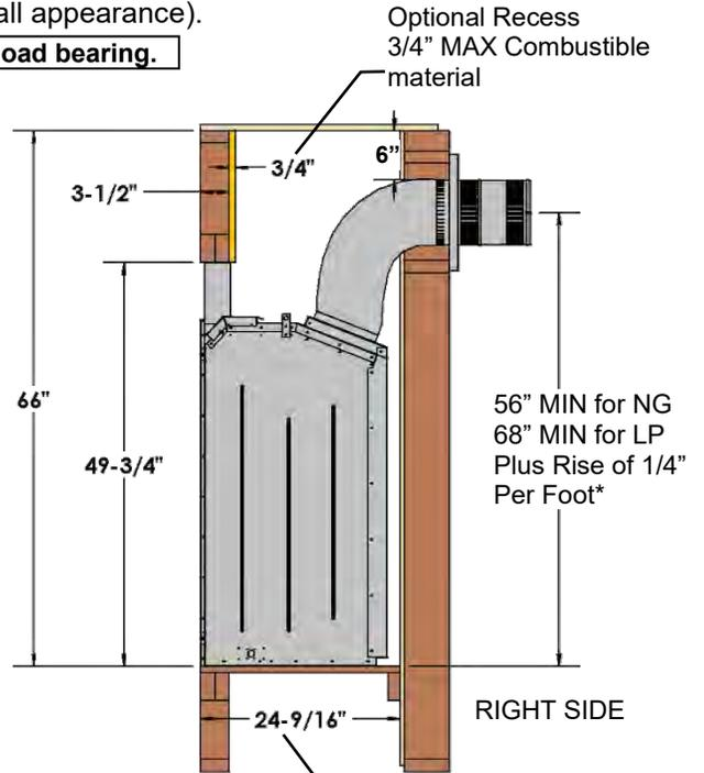
**NOTE:** Depth can be reduced to 23-1/4" if using Flex Venting
