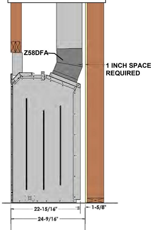
**Vent Framing (Vertical or Horizontal) 9" Round Hole through Masonry. 12" x 12" Framing for Combustible.**
