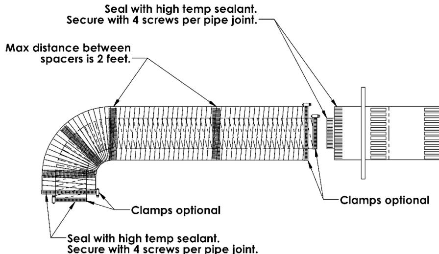
1. To determine the minimum distance from the bottom of fireplace to center of vent see the **Framing Your Gas Fireplace** section. Cut a hole through the wall allowing for a 12" x 12" (inside diameter) in combustible walls for wall thimble or a 9" diameter hole in a non-combustible wall (See Figure 2).
