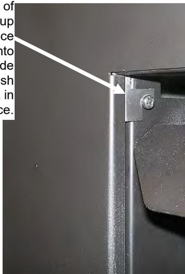
**3.** Swing Lower Tab Mount into frame of fireplace below Access Panel support bracket. Insert screws and tighten. Replace Access Cover.
