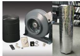
An optional 635 cfm external blower can be used to circulate the heat from the fireplace in any direction. The kit includes a 5 ft. length of acoustic ducting, a variable speed control, a mounting bracket and a back draft damper. Can be installed on the left side only.
