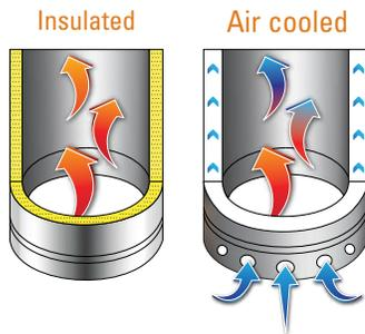
**High efficiency fireplaces are wood stoves** with cabinets around them to keep the outside of the cabinet cool and circulate the stove’s heat into the room. They warm up faster, draw better and form less creosote when they are installed with an insulated chimney. That’s why RSF Fireplaces are only approved with Excel insulated chimney, which passes ULC S-629M, the most stringent chimney safety standard in North America.
