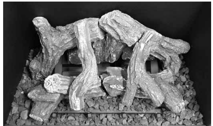
STEP 5: Place glowing embers on the front of the burner tube and ember plates. Place lava rock and vermiculite on the burner pan as shown. DO NOT PLACE LAVA ROCK AND VERMICULITE ON BURNER TUBE.
