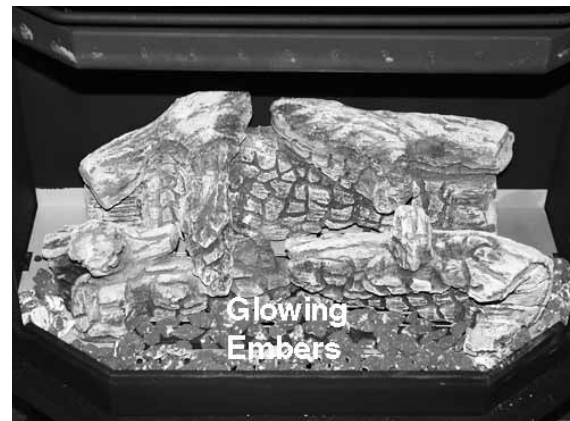
A bag of Ember chunks is supplied with the log set, it is very important that these chunks are placed onto the front burner and log mounting pan as shown in the picture, spread the ember chunks out no more than on Layer deep. NOTE: IF YOU DO NOT FOLLOW THIS INSTRUCTION CORRECTLY SOOTING PROBLEMS CAN OCCUR.
