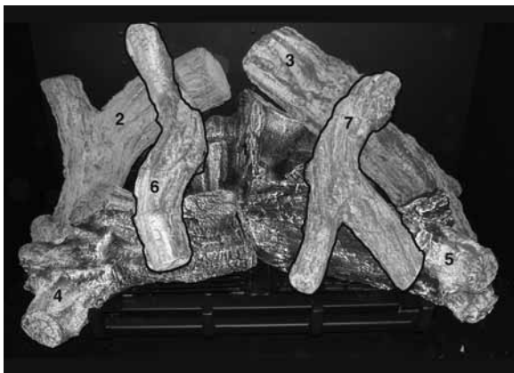
Locate 1 hole bottom of Log #6 and place onto pin of Log #2. Locate 2 holes bottom of Log #7 and place onto pins of Log #5.
