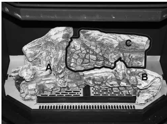
Log C has to be lowered into position just behind logs A and B. Log C has an area notched out of the rear of it to fit over rear positioning bracket as shown in the picture.
