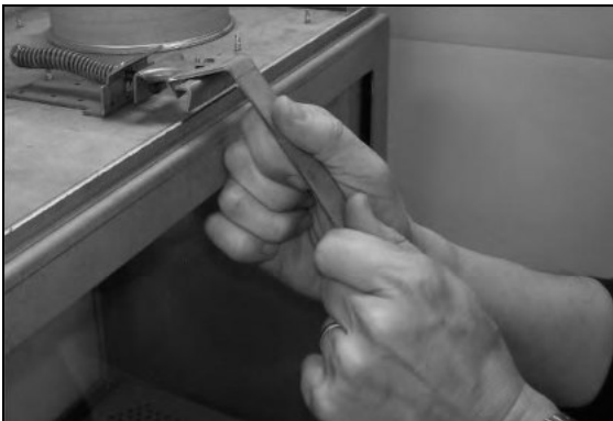
Step 5: Release Latch from Door.
