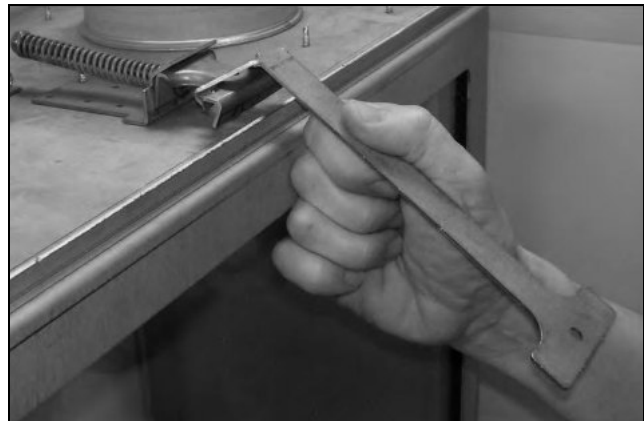
Step 6: Release Tool from Latch.
