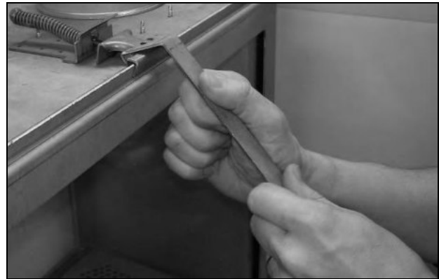
Step 4: Draw Latch forward with other hand.
