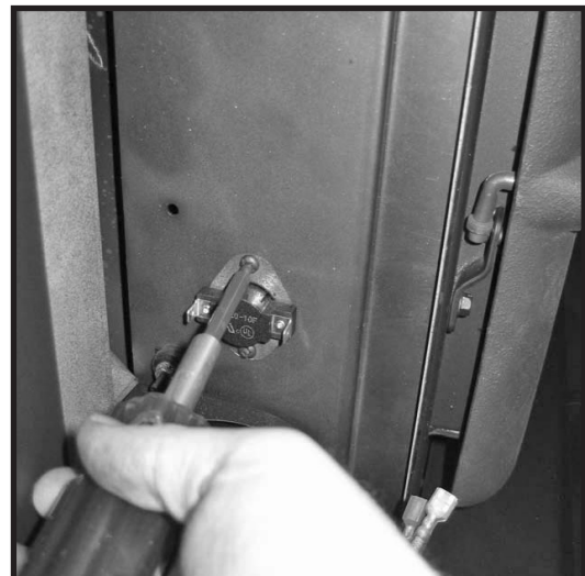
Figure 21: Relocating thermal switch to left side.
