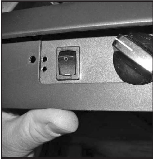
Figure 18: Reinstalling the Speed control assy.
