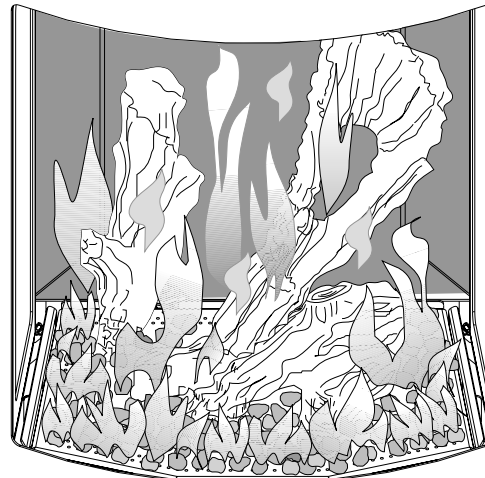
Figure 38. Proper flame picture -Traditional Logs.
