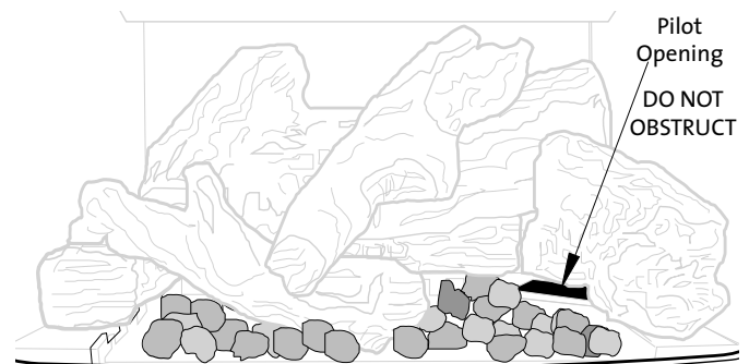
Figure 24a. Position embers loosely and maintain 1/4" clearance from the burner skirt edges.
