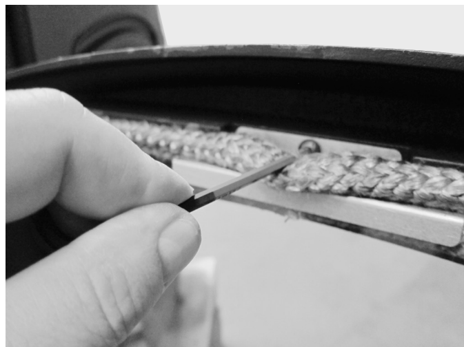
Figure 20. Loosen the glass clips.
