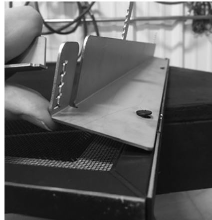
Figure 4.10, Screw Location on Hanging Bracket
